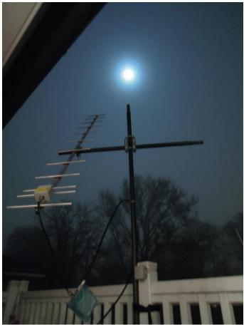
Even the smaller stations can have success in the EME contest. This single 12-element Yagi was hand-positioned on the balcony by DK1KW to make several digital EME QSOs. (Photo by DK1KW)
