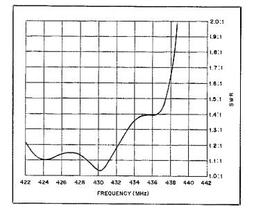
Fig 5—SWR performance of the K1FO 22-element Yagi in wet weather.
