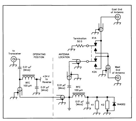
Figure 2—Relay-switching a TW antenna's pattern. RF chokes and blocking capacitors let the feed line carry the relay power.
