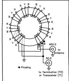
Figure 4—Winding details for the 50:450  $\Omega$  impedance transformer.
