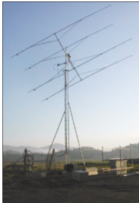
Jeremy, W7EME, used this remotely operated 2 meter array of four 17 element Yagis to monitor activity during the contest. [Photo courtesy W7EME]
