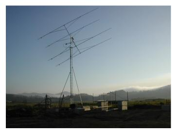
Jeremy, W7EME used this remotely-operated 2 meter array of four 17-element Yagis to monitor activity during the contest.
