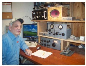
Jim, N2EY calls this 100 % vacuum-tube rig a Southgate Type 7, built in the 1990s to replace his former rig, also homebrew, called the Southgate Type 6. (Photo by N2EY)
