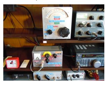
"I started hamming in the 1950s and that rig is from then," he said. "It can do five watts out on the lower bands without sweating too hard." Dan made contacts with a combination of TS-690 and Tube Tuna Tin (www.qsl.net/wd8das/T5pix.html) rigs to win the QRP category of 2014 Sweepstakes from Calgary, Alberta. When fishing for contacts, a Drake R-4C handled receive duties. His 847 contacts and 81 sections handed him the
