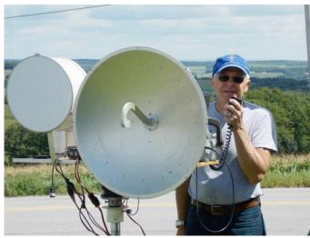
David, K2DH, operates from west of Rochester, NY at FN02xu. His setup runs 10 watts to his 10 GHz dish and 2 watts to his 24 GHz dish. (Photo K2DH)
