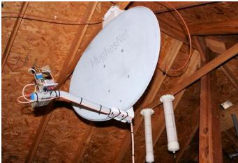
Tom, K5TRA, of Austin, TX, is able to avoid the elements with his home station. He has a dish mounted in the attic that has azimuth and elevation control. He has worked hundreds of kilometers from the comfort of home.
