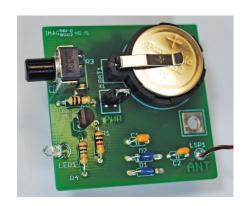
Components mount on a 1.75-inchsquare PC board. The kit can be powered from the provided coin cell battery or external power. Price: \$15. For more information or to order see www.qrpkits.com.
