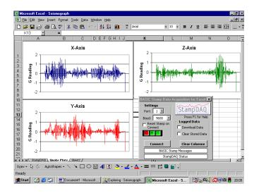
besides "shaking dirt." The Stamp could be programmed to store accelerations in ROM and then dump the data to StampDAQ. The 9 volt battery power source makes the seismometer a portable accelerometer that students can take on rides to study amusement park physics. Or the seismometer can tag along for vehicular motion studies.
