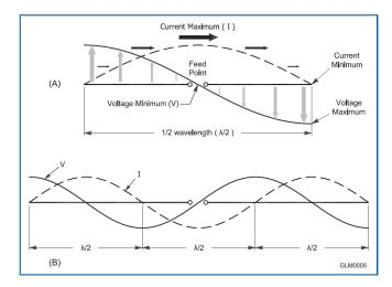
The drawing above shows the current and voltage distributions. The distributions along the wire are just the magnitude of the waveforms (like the envelope of a modulated signal) and doesn't say anything about the phase of the actual waveform. It is the distributions that are 90 degrees out of phase, not the waveforms. At the center, the voltage waveform reaches a minimum while
