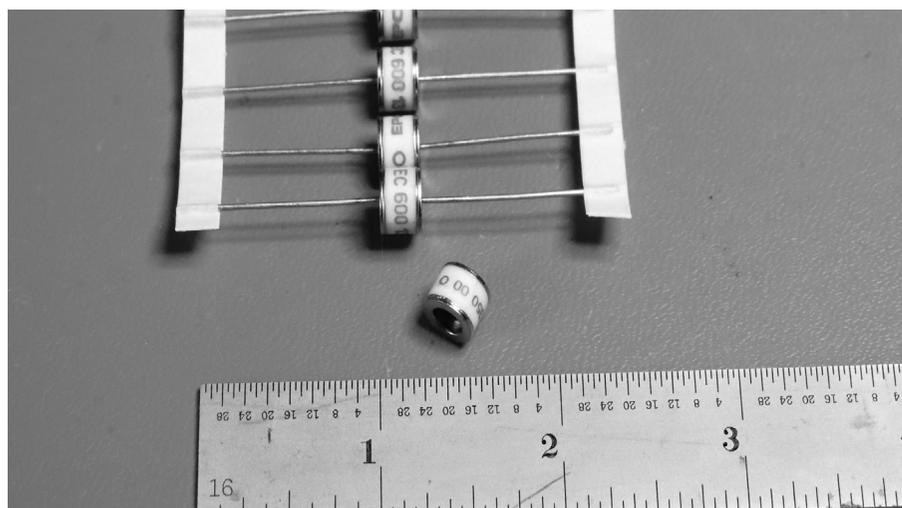
← Figure 2(a) — Axial lead format of EPCOS discharge tube.
