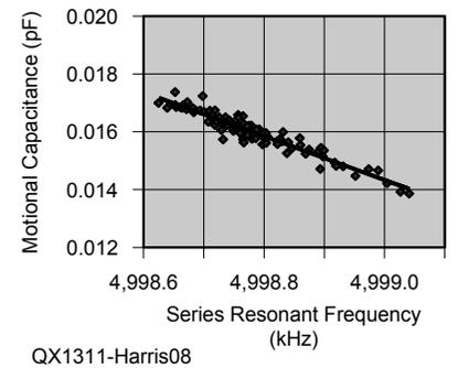
**Figure 8 — Here is a plot of the motional capacitance,  $C_m$ , versus series resonant frequency,  $f_s$ , for the batch of crystals.**
