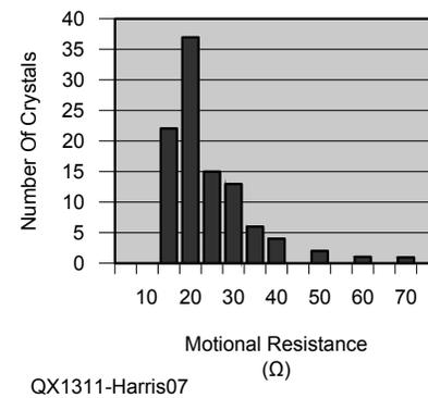
**Figure 7 — This graph shows the spread of motional resistance,  $R_m$ , for the batch of 100 crystals.**
