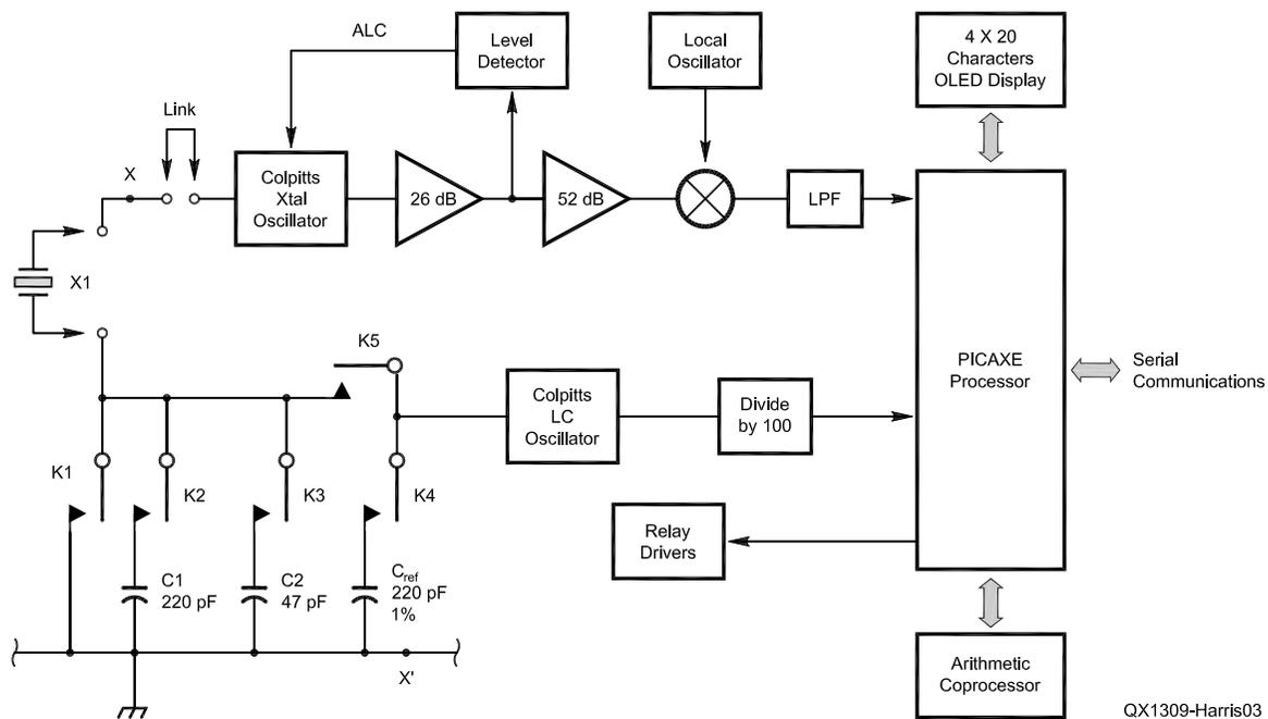
Figure 3 — The schematic/block diagram hybrid of the author's crystal measurement unit.
