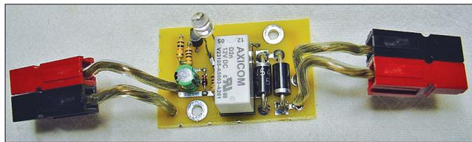
**Figure 3** — Voltage reducer prior to installation in case. The Powerpole input and output connectors are wired to the PC board with 1/2-inch #16 AWG stranded wire pigtails.
