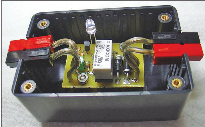
**Figure 4** — The voltage reducer mounted in a Hammond plastic box with Powerpole connectors slid into slots made with an inexpensive nibbling tool. The Reducer Enabled LED stands above the PC board to just poke through a hole in the box's top cover.
