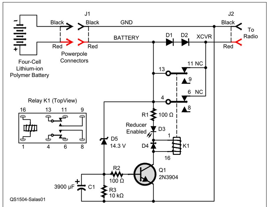
**Figure 1** — Schematic diagram of the voltage reducer. Mouser ([www.mouser.com](http://www.mouser.com)) part numbers in parentheses.
