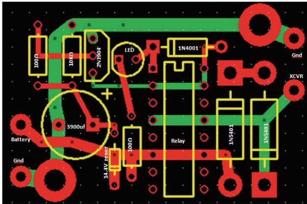
**Figure 2** — Voltage reducer PC board layout. The LED/D3 anode (long lead) is closest to the 2U3904.
