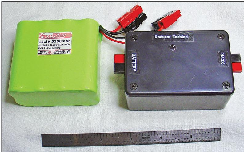
**Figure 5** — The assembled voltage reducer alongside a four-cell 5200 mAh LiPo battery. Even though the battery label lists 14.8 V, a freshly charged four-cell LiPo battery will have a voltage of 16.8 V, which is too high for most portable radios.
