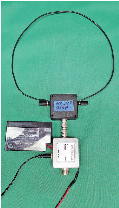
Figure 1 — An un-tuned receive-only magnetic loop, a broadband amplifier, a 12 V power inserter immediately below the pre-amplifier, and a 12 V power source (to the left) are needed, in addition to an SSB-mode receiver.
