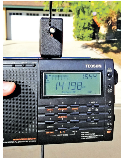
Figure 4 — Loop antenna maximum gain is in the plane (edge) of the loop, and results in the full signal strength indication on the SSB-mode receiver.
