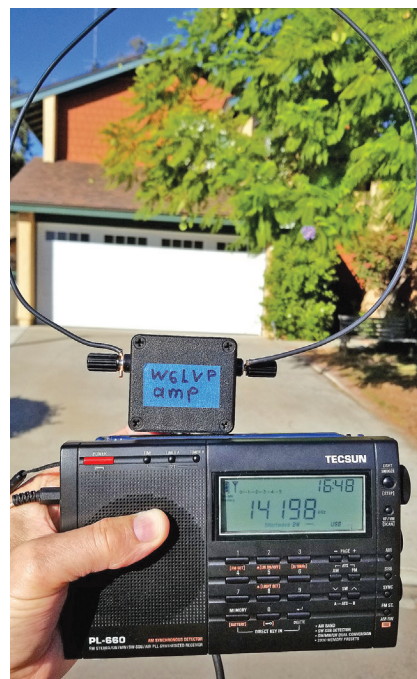
Figure 5 — Loop antenna null is on the axis of the loop and results in a zero-indicated signal strength with axis pointed toward the house.
