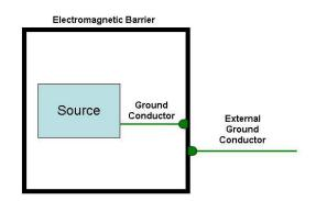
Figure 40 Barrier Treatment of a Ground Conductor
