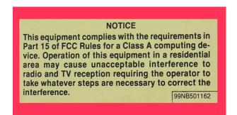
Figure 20 Radio-Interference Label from a Class A Device
