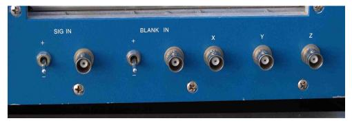
Figure 48 Coax Feed Bulkhead Connectors that Comply with BFG Principles
