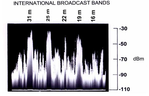
Figure 2 Example of Daytime Signal Levels in the HF Band
