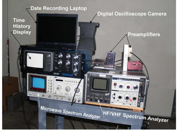
Figure 58 Typical Instrumentation configuration
