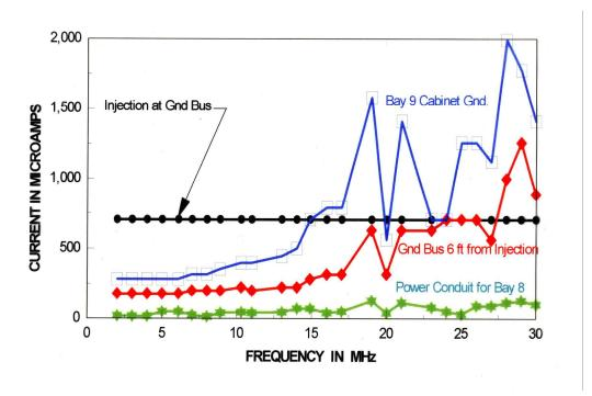
Figure 5 Standing waves along Ground Conductors
