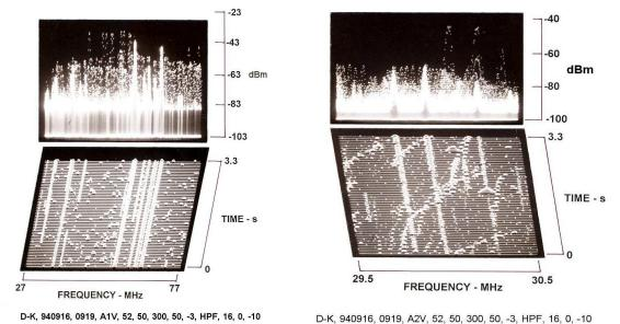
Figure 32 Intermittent Interference from Frequency-Hopping and ISM Emissions
