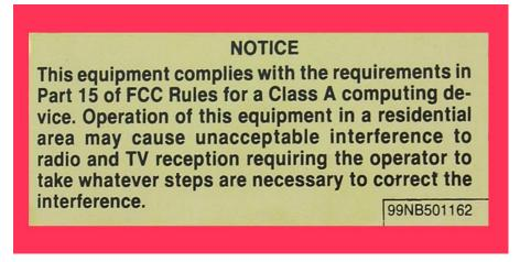
Figure 24 Example of FCC Class A Label
