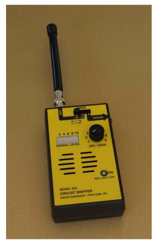
Figure 67 Circuit Sniffer Used to Locate On-Site Sources
