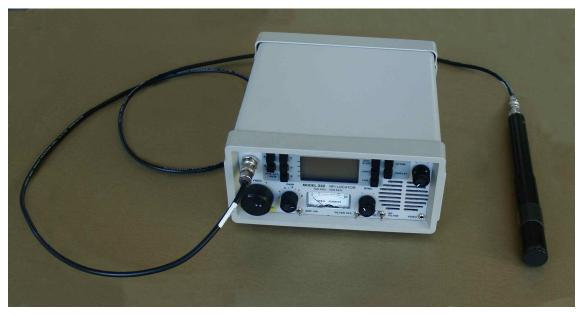
Figure 65 Radar Engineers Noise Receiver with Probe
