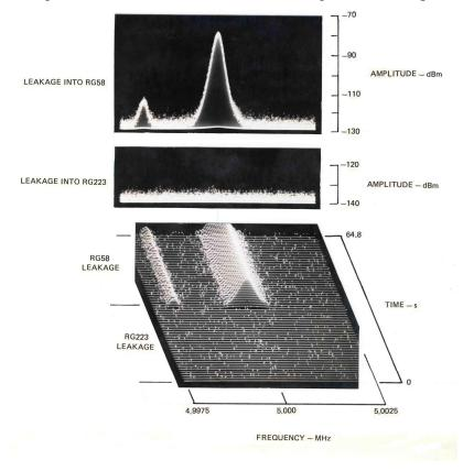
Figure 10 Example of Leakage into Coaxial Cables
