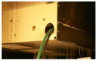
Figure 50 Unfiltered Conductors Exiting a Switching Power Supply
