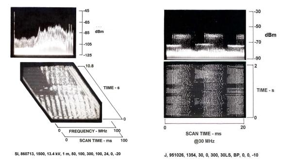
Figure 33 The Complex Structure of Intermittent Power Line Interference
