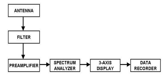
Figure 57 Block Diagram of the Instrumentation
