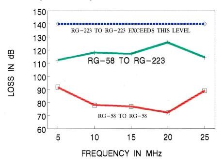
Figure 11 Cable-to-Cable Coupling Loss
