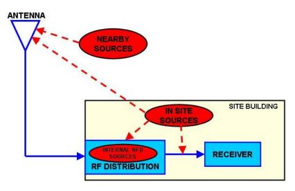
Figure 1 Block Diagram of On-Site Sources
