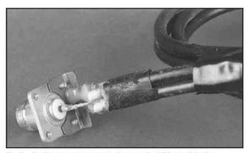
Fig 7—An N connector attached to a pair of 75- $\Omega$  cables in parallel.
