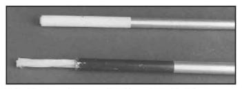
Fig 9—The element tips are painted for color-coding. The rope used to damp vibrations is partially pulled out of the lower element.
