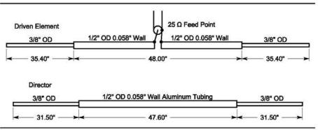
Fig 3-6061-T6 aluminum element dimensions for the 6-meter beam.
