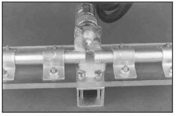
Fig 12—Dow 3140 RTV conformal coating is used to protect the feed-point connection.
