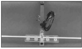
Fig 10(right) -2-turn balun made out of coiled RG-83.
