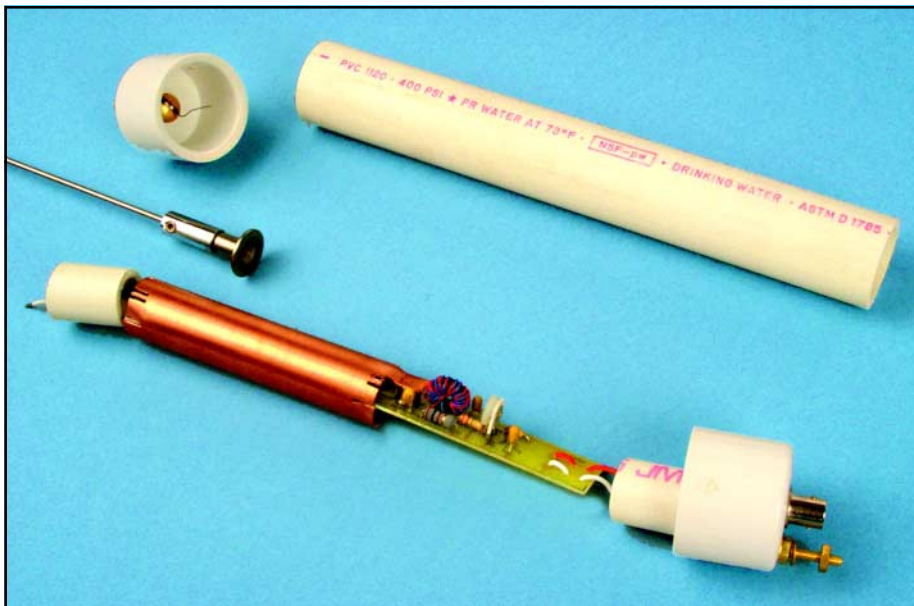
Figure 4— The amplifier, heat sink and PVC tube housing.
