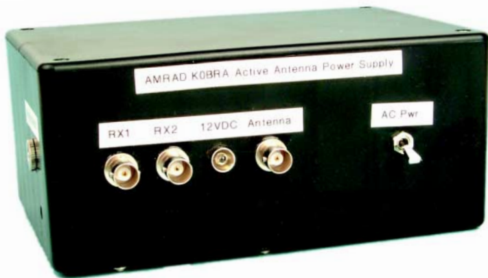
The active antenna power supply enclosure with BNC jacks for the coaxial cables to the active antenna and receivers.
