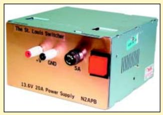
Here's the finished product. The "standard" switching power supply was removed from an old PC, doctored up in the manner described by NØXEU, and has a new "front panel" fashioned out of printed-circuit board (PCB) material. See how this was accomplished in the following photos.
