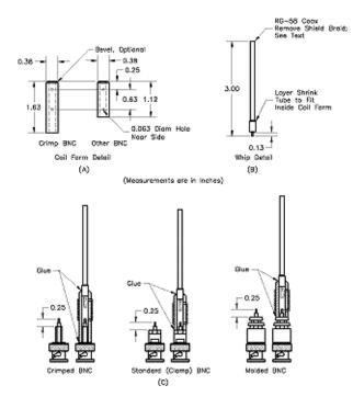
Figure 1—Making a replacement H-T antenna is relatively simple. The details show the dimensions and cross-sections of the coil form (A), whip (B), and the initial and finished stages of antennas (C) made with three types of BNC connectors: standard, crimped and molded.
