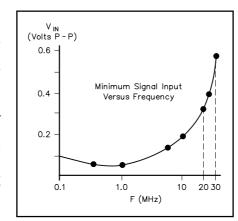
Figure 1—Input sensitivity versus frequency.
