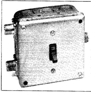
Save a few bucks in the shack—use wall-toggle switches as RF switches!
