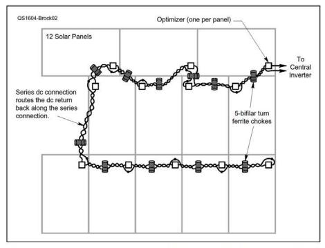
Figure 2 — New wiring configuration shows a closed loop of a twisted pair of conductors, and ferrite beads to suppress common mode currents.
