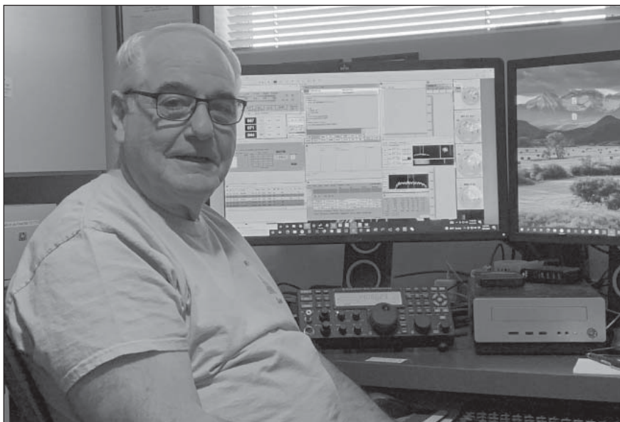
This is my operating position at home to run the NA7TB remote station 175 miles southeast of Phoenix in Safford, Arizona (DM52). I use a K3/0 Mini and a screen-sharing program. A mouse controls the antennas using Green Heron's GHE software, and the remote computer sends N1MM Logger+ CW or, in this picture, MMTTY RTTY.
