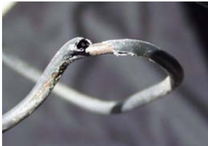
Figure 37 Insulation Failure at a Bend in a Tie Wire
