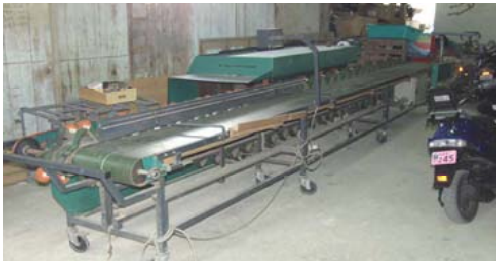
Figure 54 Photograph of Flower Processing Machine with Variable-Speed Drive
