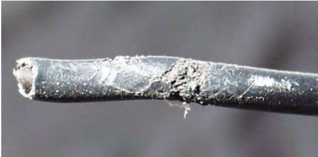
Figure 38 Insulation Failure at the End of a Tie Wire
