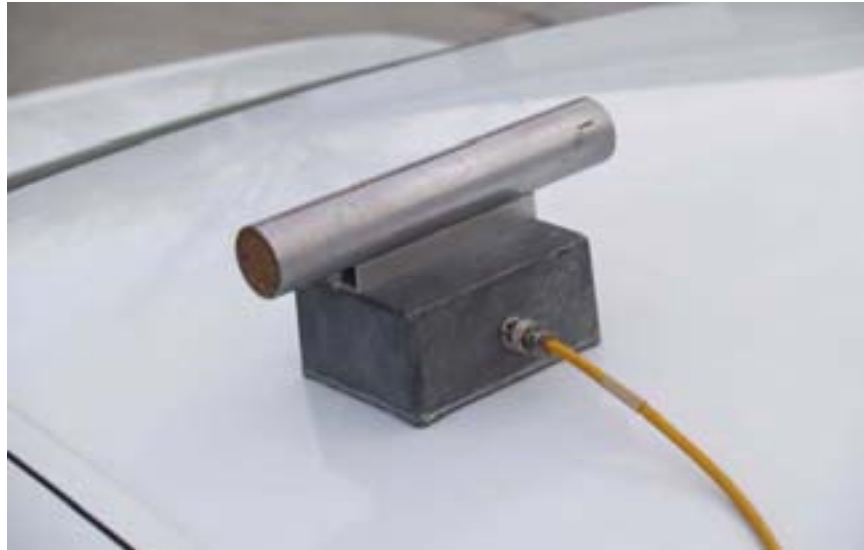
Figure 61 Loopstick Antenna on Roof of Source-Location Automobile
