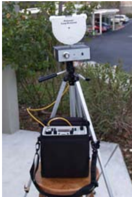
Figure 60 Loopstick Antenna for Location of Power-Conversion Sources
