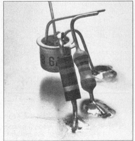
Fig 7—Once a component is firmly supported, you can make further connections without crimping. Just solder the leads as they lie side by side. This 2N5179 has its case lead grounded.
